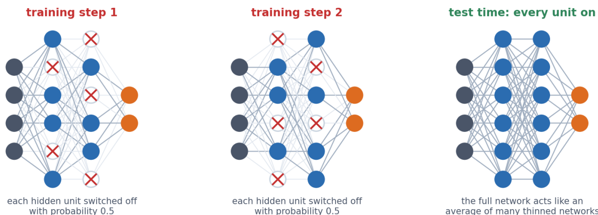
Figure 9.12: Dropout with p = 0.5 . In every training step a different random set of hidden units is switched off. At test time every unit is on.
